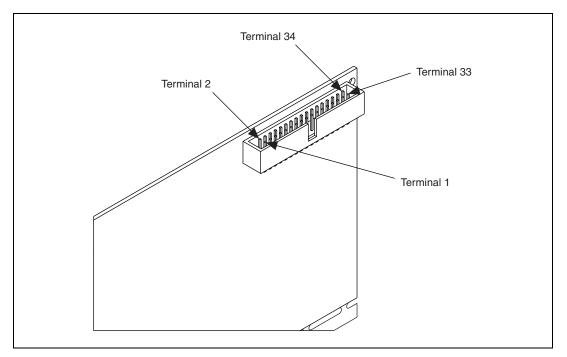
Figure 10-2. NI 6232/6233 RTSI Pinout
